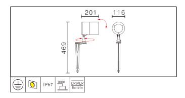
An outdoor garden spike LED luminaire featuring one high quality SHARP ZENIGATA CoB LED providing energy-efficient and low-maintenance lighting solutions. 355° rotation and 140° tilt angle to maximize lighting range. Good thermal management guarantees upto 50,000 hours lifespan.
