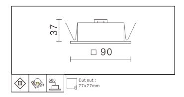
Clean-cut design indoor wall-recessed LED luminaire featuring single high quality OSRAM GD PLUS LED providing energy-efficient and low-maintenance lighting solutions. Completed with steel recess box for easy maintenance and servicing.
