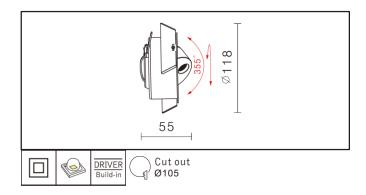
Unique design indoor wall-recessed LED luminaire featuring single high quality OSRAM GD PLUS LED providing energy-efficient and low-maintenance lighting solutions. Designed for bed side reading lamp and able to flip 180° tilt to maximize lighting range.
