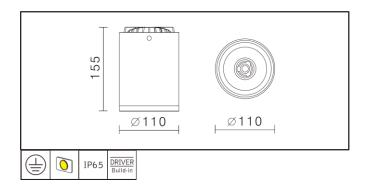
An IP65 outdoor surface-mounted luminaire featuring SHARP ZENIGATA CoB LED providing high energy saving and low maintenance cost. With protection glass on the front, easy to maintain and clean. Designed with easy wire-through function and good thermal management guarantees long lifespan.
