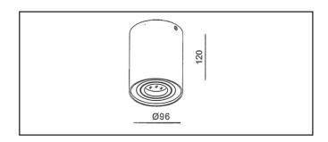
A surface-mounted LED luminaire features single halogen MR-16 or GU-10 module, suitable for various halogen lamp-source and LEDs. Easy maintenance to remove lamps after installation.
