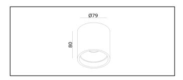
A surface-mounted luminaire features SAMSUNG AC4W LED providing energy-efficient and low-maintenance lighting solutions. General/Accent lighting for concrete and false ceiling for residences, commercial and retail applications.
