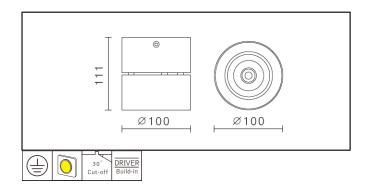
Simple and clean design surface-mounted luminaire features CREE CoB LED providing energy-efficient and low-maintenance lighting solutions. Available in two shapes; round and square, with built-in driver and easy installation process.
