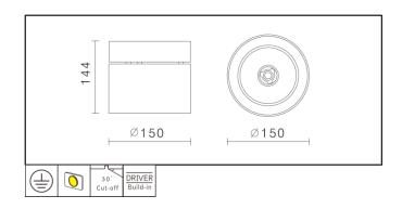
Simple and clean design surface-mounted luminaire features SHARP ZENIGATA CoB LED providing energy-efficient and low-maintenance lighting solutions. Available in two shapes; round and square, with built-in driver and easy installation process.
