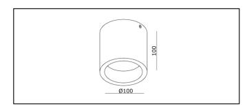
A surface-mounted luminaire features SHARP ZENIGATA CoB LED providing energy-efficient and low-maintenance lighting solutions. General/Accent lighting for concrete and false ceiling for residences, commercial and retail applications.
