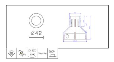
An IP67 in-ground luminaire features one high quality OSRAM OSLON LED providing energy-efficient and low-maintenance lighting solutions. Outdoor floor-recessed illumination for foyers, pathway, garden and park.
