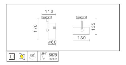
Clean and classy design LED track luminaire features SHARP ZENIGATA CoB LED providing energy-efficient and low-maintenance lighting solutions. 180° tilt angle to maximize lighting range. Replacement of conventional MR-16 track luminaires, etc.
