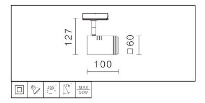
Clean and classy design track luminaire features a wide range of lamp sources; Halogens and LEDs.  $355^{\circ}$  rotation and  $90^{\circ}$  tilt angle to maximize lighting range.
