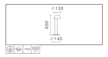
An IP65 outdoor bollard with three high quality OSRAM SQUARE LED providing energy-efficient and low-maintenance lighting solutions. Anti-dazzle design ensures visual comfort and patent thermal application guarantees a long lifespan.
