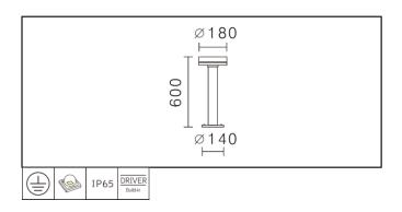
An IP65 outdoor bollard with six high quality OSRAM OSLON LED providing energy-efficient and low-maintenance lighting solutions. Anti-dazzle design ensures visual comfort and patent thermal application guarantees a long lifespan.
