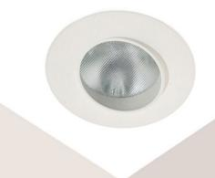
The Mini Wall Wash Snoot was developed with a well-known UK lighting designer as a special project solution. To achieve best wall-washing effect we recommend these are installed 600mm from walls and 1.0-1.2m apart.
