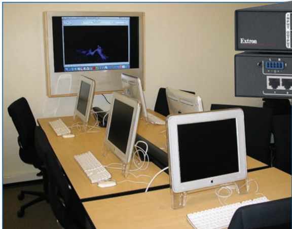
Above: The Extron TPX 88 A Twisted Pair Matrix Switcher with Audio was chosen due in part to the very limited space available.
