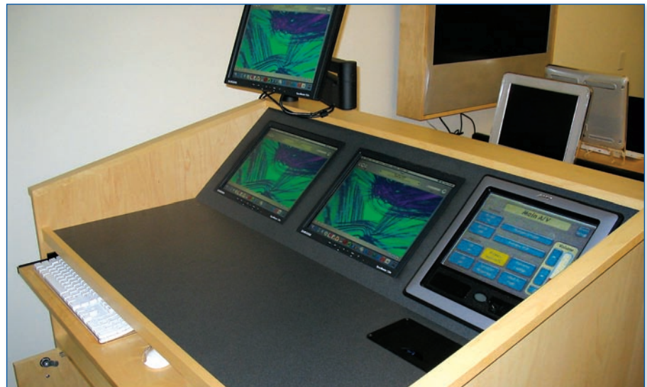
Above: The computer lab lectern includes a touch-screen, computer monitors, and an Extron Cable Cubby 200. Left: Classroom system control and connectivity are easily accessible using the MediaLink Controller.
